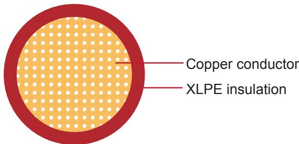
**Conductor:** Annealed stranded copper (Type B)
