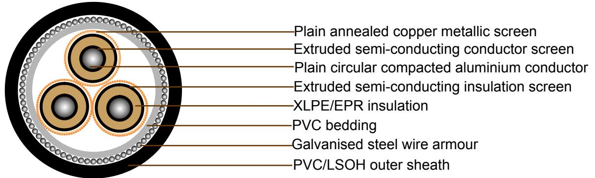
**CONDUCTOR:** Plain circular compacted aluminium to AS/NZS1125
