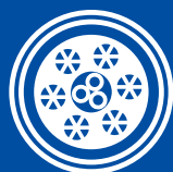
Fig 8 Solid PE Insulated & AP Sheathed (Alpeth) Air Core Cable to ICEA S-85-625
